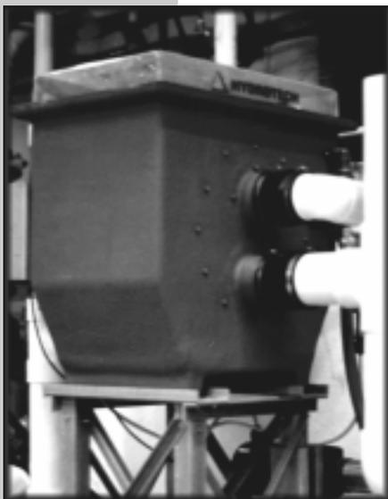
Hydrotech Filter 501 - Flow Rate= 132 gpm
